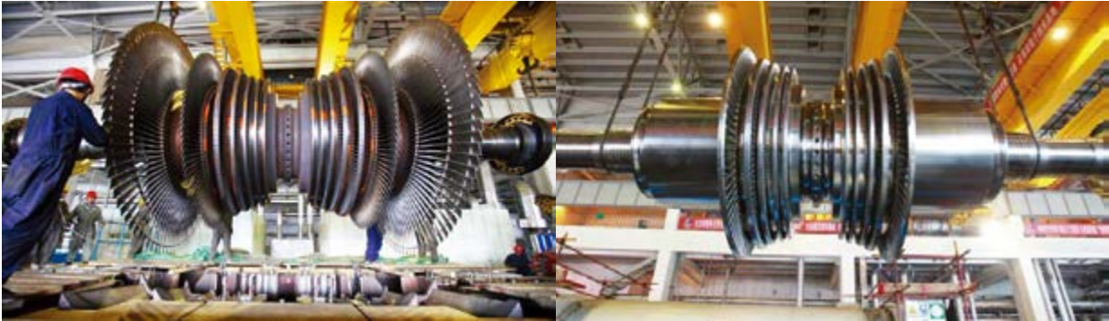
图 2 135MW 机组新、旧低压转子照片 Figure 2 Pictures of the new and the old low-pressure rotor
