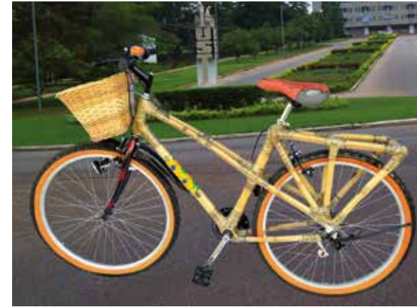
Female Mountain Bike with diagonal stays and rack 带有对角拉撑和行李架的女性山地自行车
