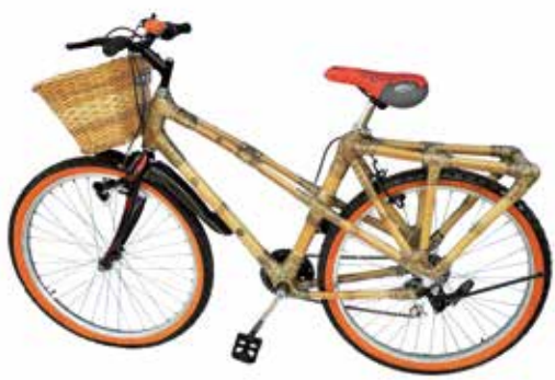
Female Mountain Bike with diagonal stays and rack 带有对角拉撑和行李架的女性山地自行车
